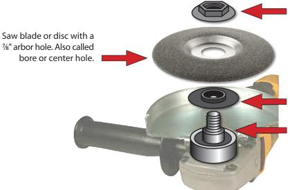
%"–11 threaded nut included with tool. Also called disc nut, clamping flange, etc.
